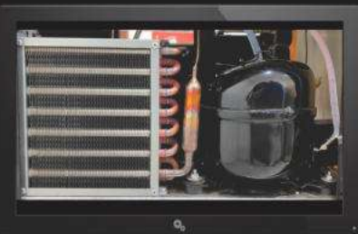
SMALL COMPRESSOR SYSTEM (Pre Cooling)
