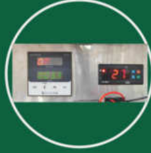
JUICE OUTPUT COUNTING SYSTEM WITH (ML) SETTING AND COOLING TEMPRETURE CONTROLLER
