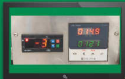
JUICE OUTPUT COUNTING SYSTEM WITH (ML) SETTING AND COOLING TEMPRETURE CONTROLLER
