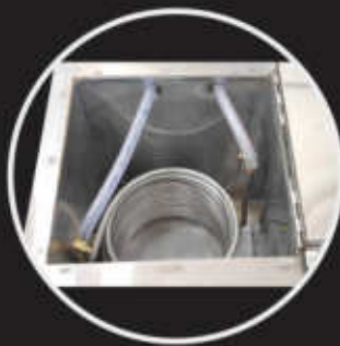
ICE STORAGE TANK
