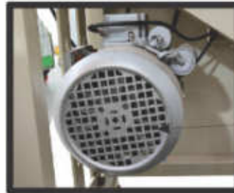
1 HP MOTOR (COPPER WINDING)
