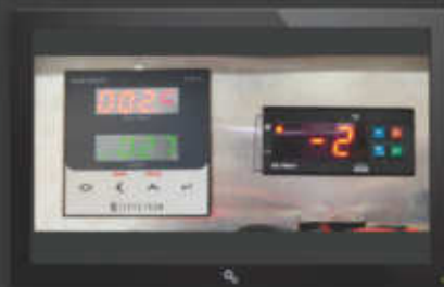
JUICE OUTPUT COUNTING SYSTEM WITH (ML) SETTING AND COOLING TEMPERATURE CONTROLLER
